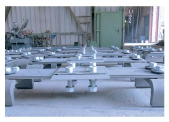
The benefit is that the system includes in-built thermal protection. Depending on the clearance between the kiln shell and the girth gear, single or double thermal protection is provided. This protects the girth gear from excessive heat radiation from the kiln. The periphery deserves particular consideration with the use of secondary fuels and higher process temperatures, or with regard to shifting of the clinkering zone.
