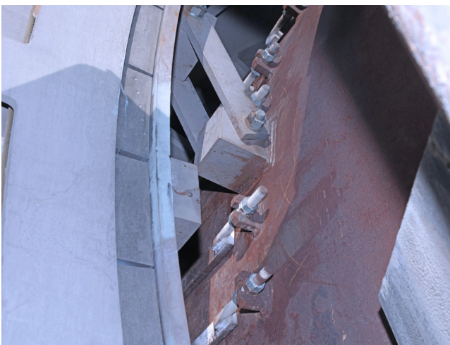
The tangential support on the kiln outlet side facilitates assembly if kiln shells are deformed – independent of the kiln manufacturer.
