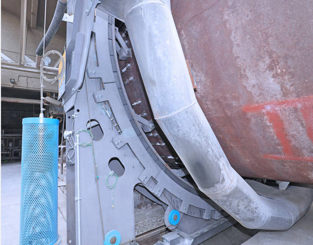
Two separate tensioning ropes for the upper and lower strand ensure easy and uniform pretensioning by steel weights.
