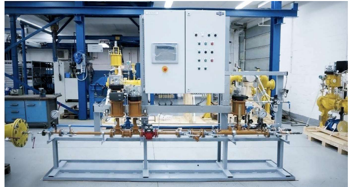
Burner operating valve station/Valve station for oil
