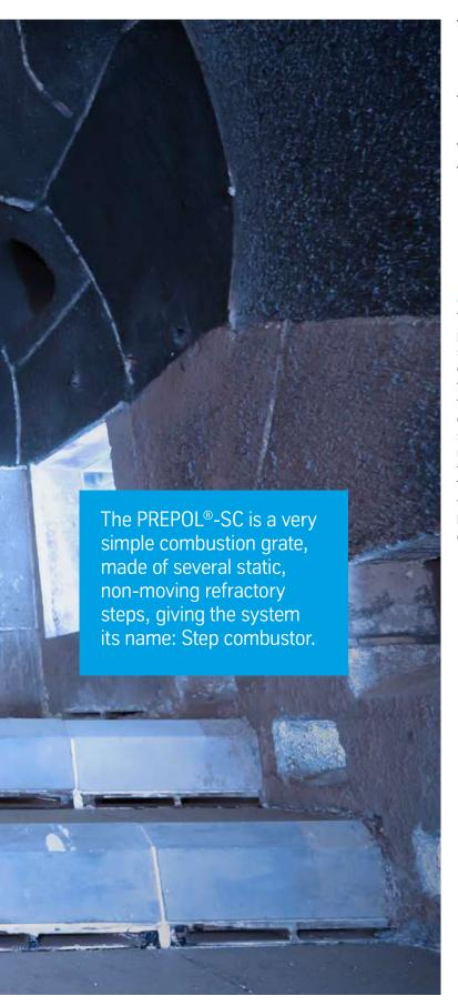
The PREPOL®-SC is an add-on for the PREPOL® precalciner. On this simple combustion grate, waste can burn for more than 1,000 seconds at high temperatures. Compared to ordinary calciner technology with only up to 7 seconds residence time the PREPOL®-SC opens a new dimension in combustion: New sorts of wastes can be utilized resulting in a new level of fuel-cost savings.
