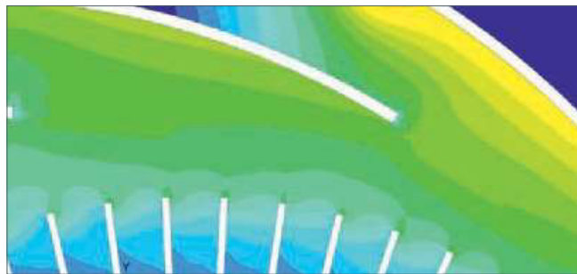
Optimum air distribution thanks to curved guide vanes
