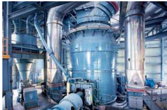
A QMC 2 -RD mill in France producing OPC finenesses < 10% R 25 µm.
