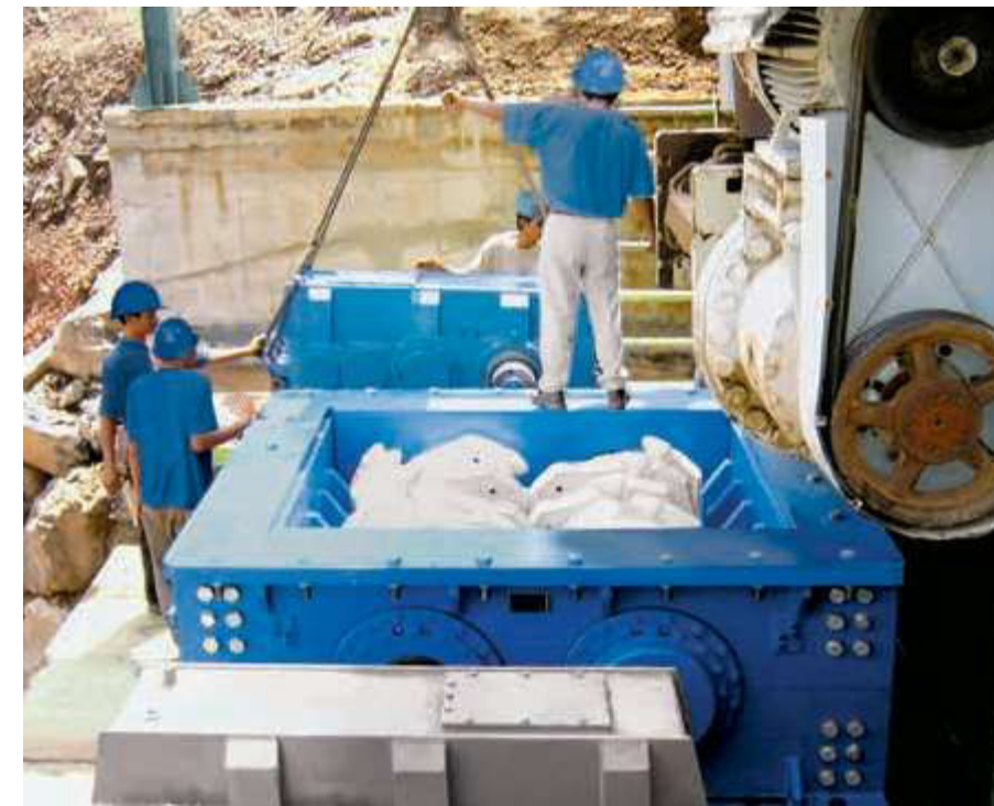
RollSizer, DRS 800 x 1500 CenterSizer, for the primary crushing of silicate rocks. Throughput rate: 700 t/h
