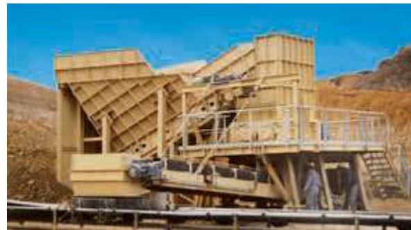
Semi-mobile RollSizer crushing plant, DRS 660 x 1500 CenterSizer, for the primary crushing of limestone. Throughput rate: 550 t/h
