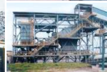
Semi-mobile impact crusher plant at Loma Negra S.A., Olavarria, Argentina Type PB 220/300 Throughput rate 2,200 t/h
