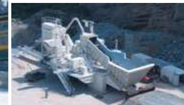
Semi-mobile impact crusher plant at Jura Cement, Wildeg, Switzerland Type PB 180/200 CR Throughput rate 700 t/h <80 mm 250 t/h <35 mm
