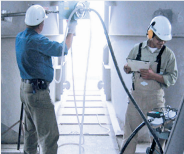
Dust measurement in the preheater
