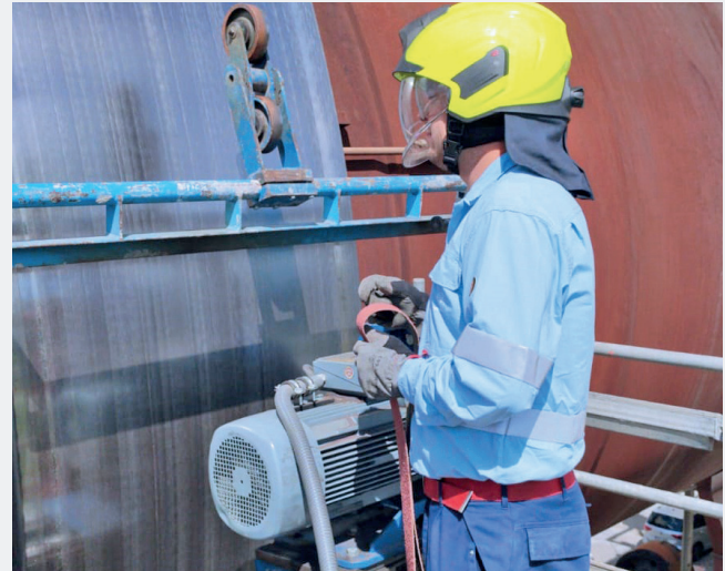
Our polgrind® service ensures your tyres and supporting rollers are trued up again.
