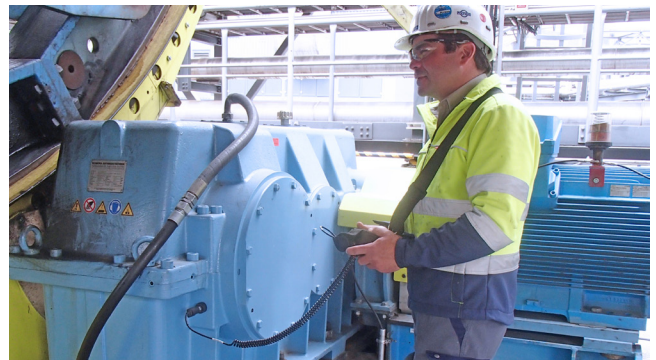
Vibration measurements on a spur gear unit
