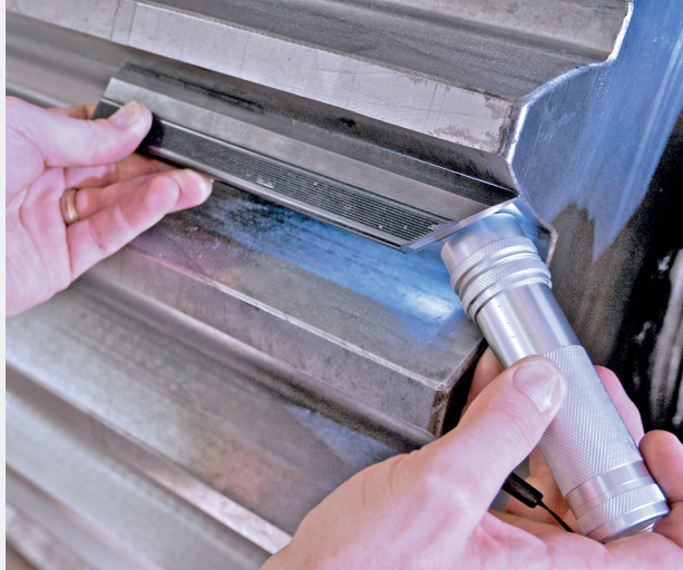
Wear inspection at the loaded flank of large tooth gearing
