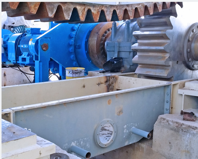
Assembling the oil sump of a double pinion drive
