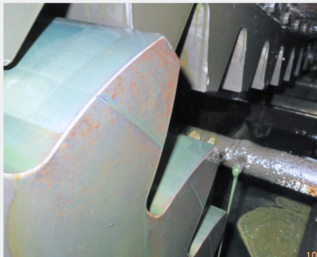
Oil distribution with an inward-running pinion
