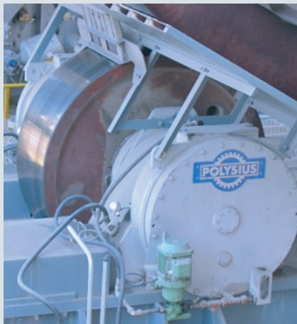
Supporting roller in operation
