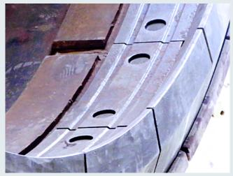
In the case of thyssenkrupp kilns, the new protective segment can be used to replace the original component.
